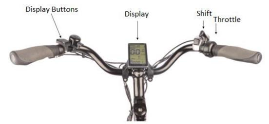
The following parts on the handlebar will help you understand how to safely operate this bike.
