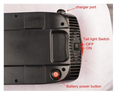
To activate the bike battery, you need to insert the battery in the slot, turn the key on the battery to the lock position and press the battery power button once.
