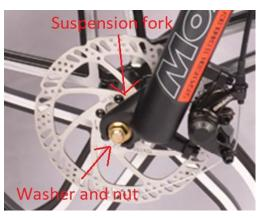
• Put a washer and a nut on each side of the wheel axle
