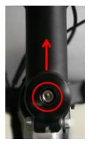
• If the Allen bolt on top of the handlebar is not visible, use the wrench to unscrew the bolt and turn the handlebar post 180°. The bolt should be below the handlebar
